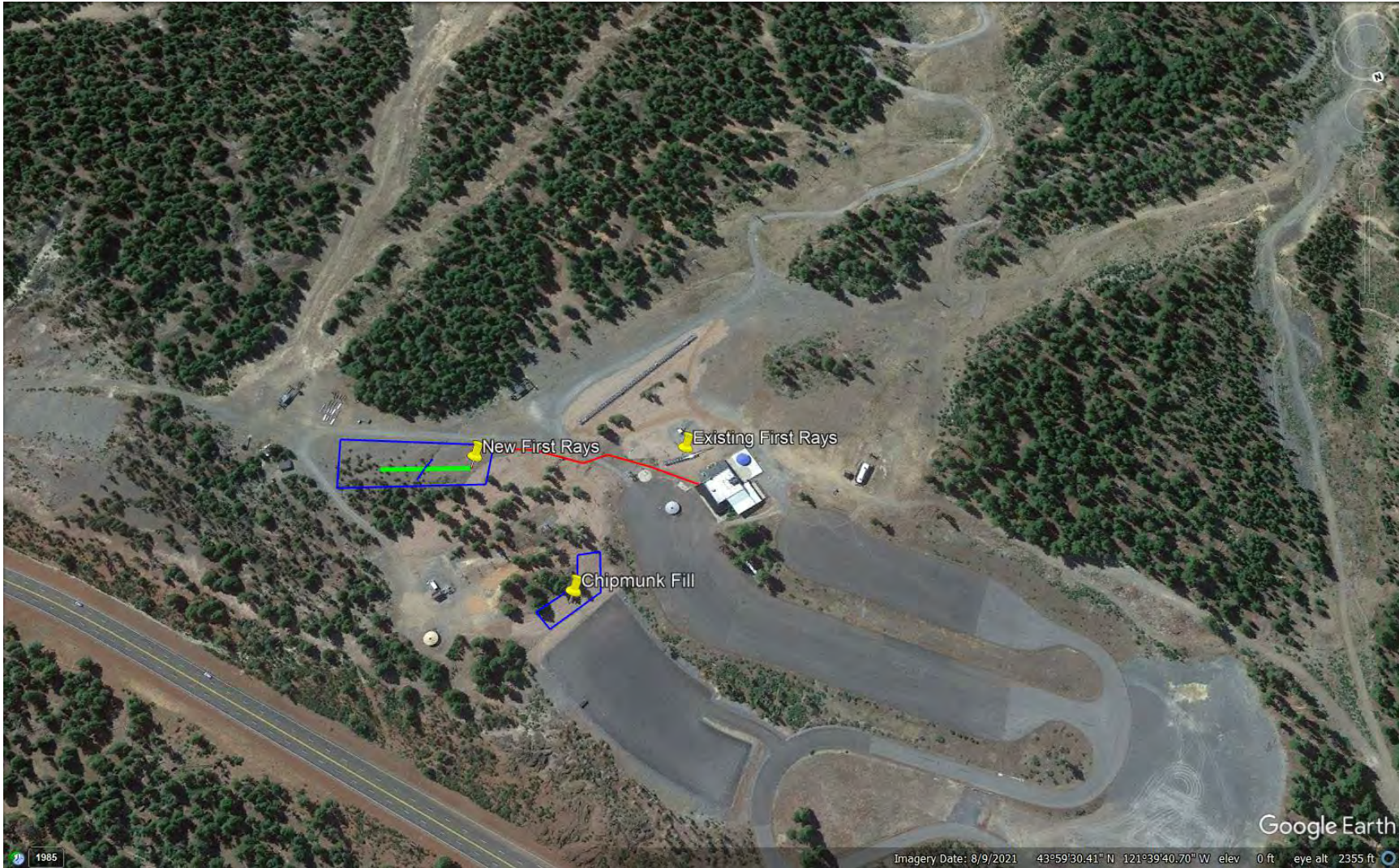
Figure 5. Surface Lifts Improvements for First Rays Carpet showing new location (green), lift tower location (blue), power trench (red) and Chipmunk fill disposal area.
