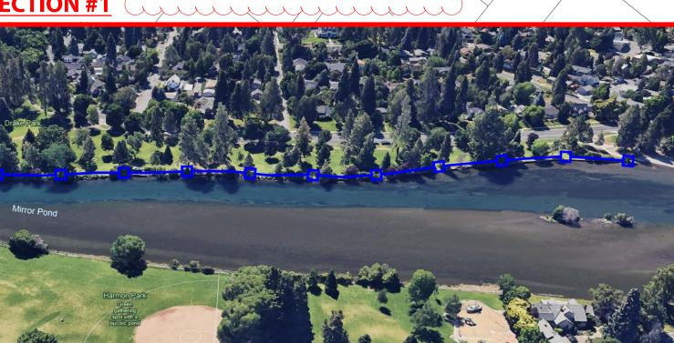
46" (2) RAIL CEDER SPLIT RAIL FENCE PER BPRD DEVELOPMENT STANDARD DETAIL - INSTALL ALONG BACK EDGE OF EXISTING RIVER WALL, MEANDERING TO AVOID **EXISTING TREES AND SHRUBS**
